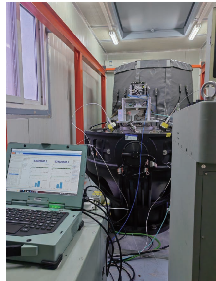
Photo of the marine gravimeter field calibration device during offshore testing
