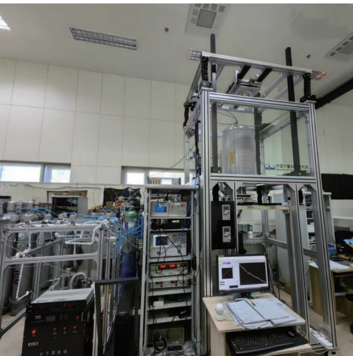
Integrated primary acoustic gas and radiometric thermometer with same temperature source
