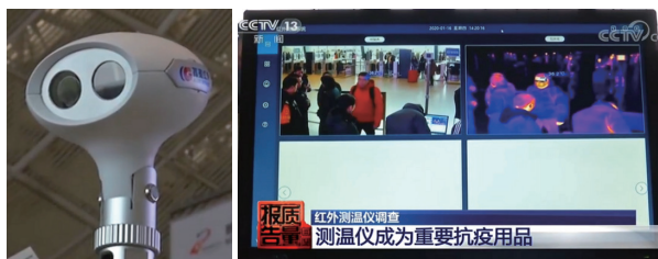
Fig. 3 A thermal imager for fever screening with its application
