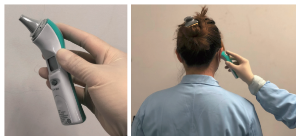
Fig. 1 An infrared ear thermometer with its application
