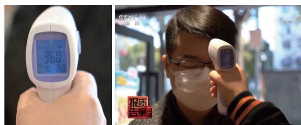
Fig. 2 An infrared forehead thermometer with its application
