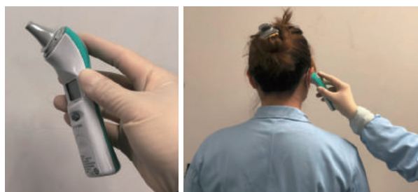
Fig. 1 An infrared ear thermometer with its application
